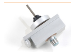
Tool 8: Linear Abrader "Crockmeter" (200g/7.05oz)
