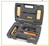
technique and has been designed to set a new standard got wet sponge detectors — a high quality, low voltage detector with similar accessories to a high voltage spark tester.
