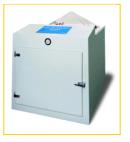
resistant coatings are to corrosion. It provides a mist of brine in controlled conditions of humidity and temperature. These conditions promote rapid rusting of steel exposed by a cut through the coating.
