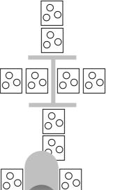
Beams (left) have two Reference Areas per metre length, both on the web (middle part) and on the flanges (top and bottom part).
