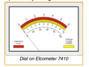
there are no complicated conversion calculations or confusion over which scale to read, making your job quicker and easier. Simply switch on the gauge, press against the surface and take a reading from the dial.
