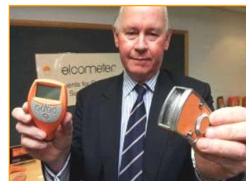
The digital Elcometer 456 (left) developed from the original "Elcometer" (now 101), which had no electrical parts.
