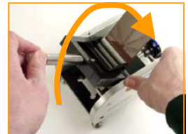
Small panels over small cylinders, bent as the lever is moved left to right
