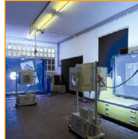
Ultra-violet light hardening the light sensitive emulsion
