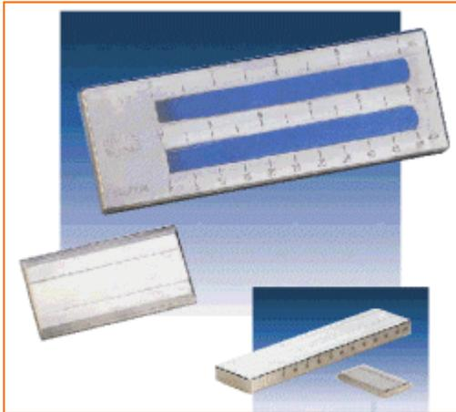
Elcometer 2020 & 2041 Grindometer – Hegman, North & PCU
