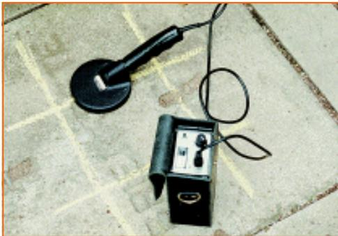
Elcometer P100 Imp Rebar Locator
