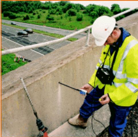
Elcometer Borehole Probe / Tendon Duct Locator
