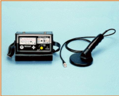
Elcometer P120 Rebar Locator
